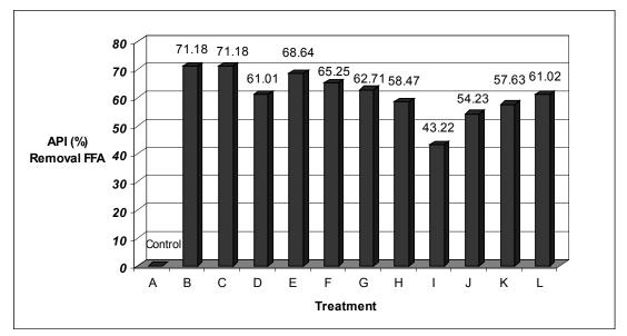
Figure 3. The percentage removal of FFA using adsorbent with various levels of Magnesol XL treatment
